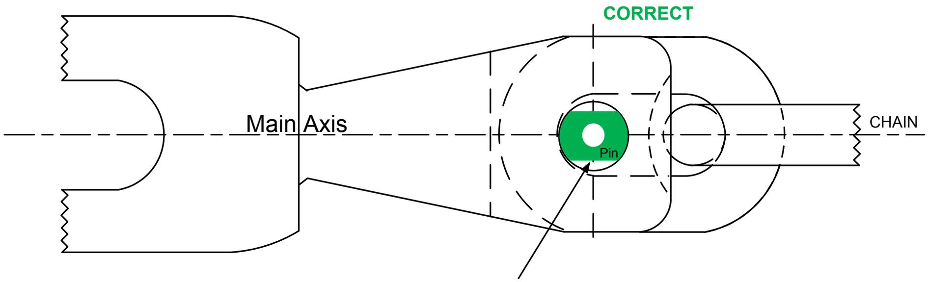
Flat surfaces of the pin must be connected parallel to the Main Axis
