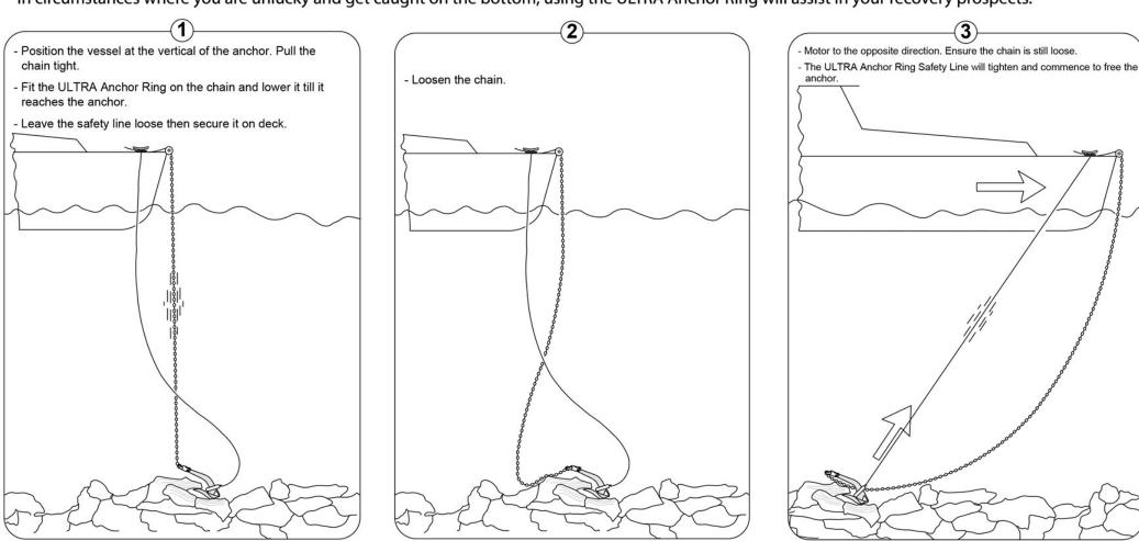
Note: If the chain itself is fouled, deploying the ULTRA Anchor Ring and applaying the same procedure is possible.
