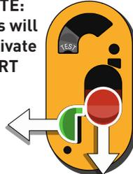
4 Whilst holding the red switch down, release the green switch to lock in active position.
