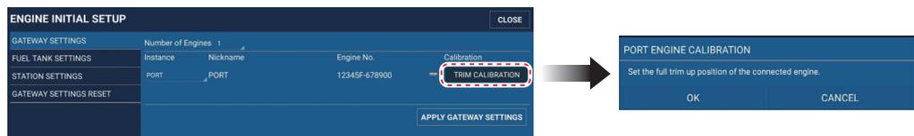
2. Set the full trim up position of the connected engine, then tap the [OK] button. The following message appears.
