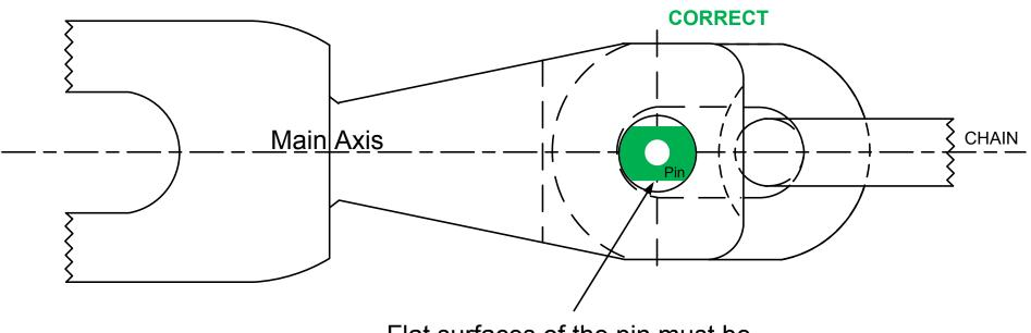
Flat surfaces of the pin must be connected parallel to the Main Axis
