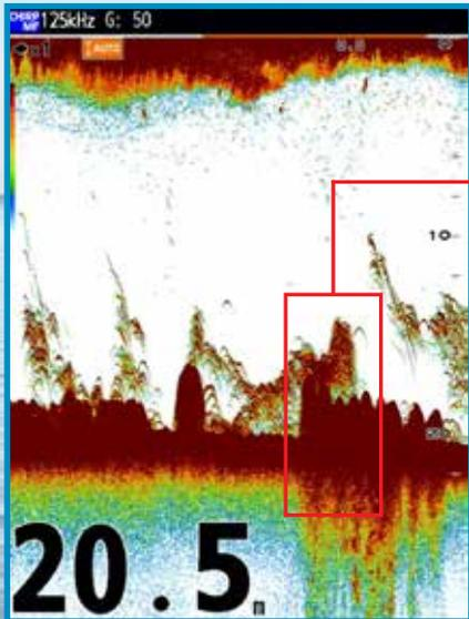
With the conventional color ranges, echoes from the seabed and a large fish are shown in a similar color, making it challenging to distinguish large fish from the bottom.
